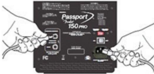
5. Connect each of your microphones, instruments and other sound sources into separate channels using the appropriate type of input jack. Use the mono channels on the left for monophonic sources such as microphones and use the stereo channels on the right for stereo/mono sources such as CD players, MP3 players, keyboards and other line level audio devices.
