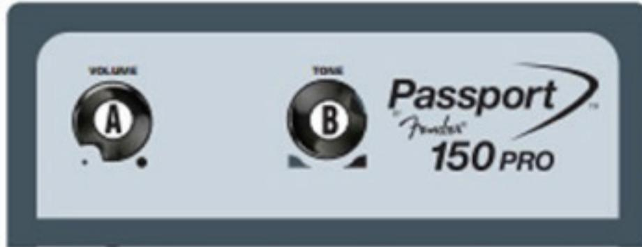
**A. VOLUME** - Use to adjust the overall loudness of your Passport Pro. When this knob is rotated fully counter-clockwise, there will be no sound coming out of the Passport speakers.
